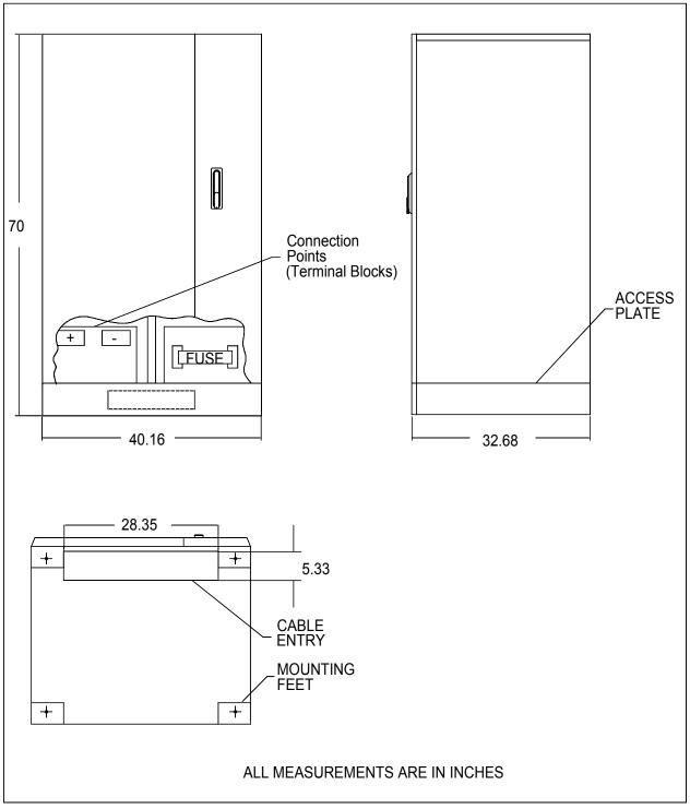
Figure 15 – "D" Battery Cabinet Drawing for 50/80kVA Ratings
